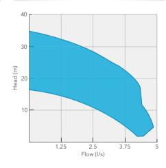
The 3069 model is now available with our patented Adaptive N technology, well tested in thousands of installations. Normally available on larger N pumps, this state-of-the-art technology not only prevents clogging and reduces stress on the shaft, seals and bearings, but it enables up to 25% sustained lower energy usage. You can also choose from different impeller material options: Hard-Iron, grey iron or stainless steel.
