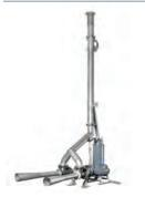
DESIGN: submersible self aspirating jet aerator TYPE: JA112, JA117, JA217 and JA317 CAPACITY: 60 kg O2/h at 7,5 meter water depth NUMBER OF EJECTORS: 1, 2 or 3 EJECTOR TYPES: 4812 (55 mm nozzle) 4817 (95 mm nozzle) N-PUMPS: 3085, 3102, 3127, 3153, 3171 and 3202
